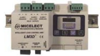
In addition, with up to eight individual sensors attached via USB connectors, the LCD display allows the user to view the individual tension in metric units for up to eight wire ropes (the field technician can then quickly and accurately equalize the rope tensions). The unit can also signal that a rope has broken and it permits the weight of the cab to be conveniently and precisely measured.
