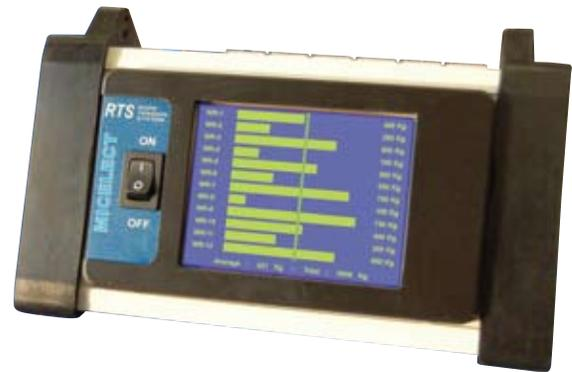
The weight of the cab and counterweight can also be conveniently and precisely measured with the RTS.
