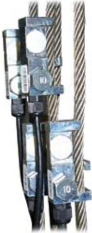
**The MWR-8 intelligent wire rope sensor system** has been developed as a load weighing device for permanent installation on elevators which require a high level of precision (within an accuracy of 5%). This is accomplished through the use of an individual sensor on each rope to measure the tension (indicate rope diameter and quantity of sensors from 2 to 8 per control unit when you place your order). Each sensor has a maximum capacity of 2200 lbs • 1000 kg.
