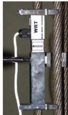
metric units for up to 12 ropes. The clearly displayed tension information allows the field technician to quickly and accurately equalize the rope tensions. Since the information is displayed in real time for each rope, the impact of a tensioning adjustment made to one rope is immediately visible on the other ropes.
